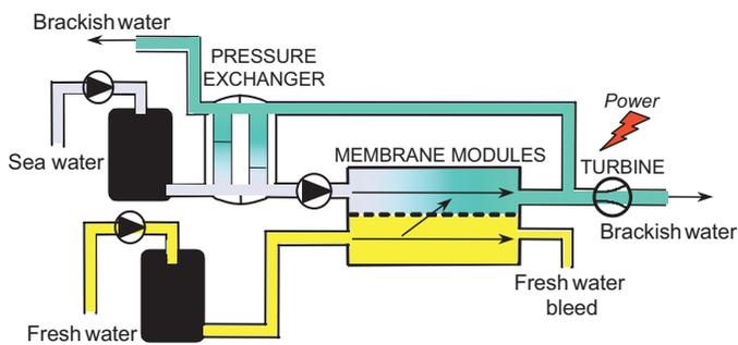
Figure 1: Simplified diagram of the PRO process.
