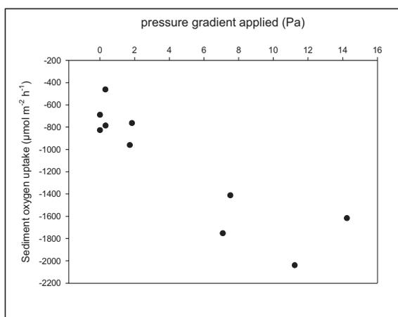
**Figure 1.** measured rates of oxygen consumption in pressure calibrated benthic chambers. *O<sub>2</sub> consumption in sandy sediments increases with rates of advection (water flow) through the sediment.*
