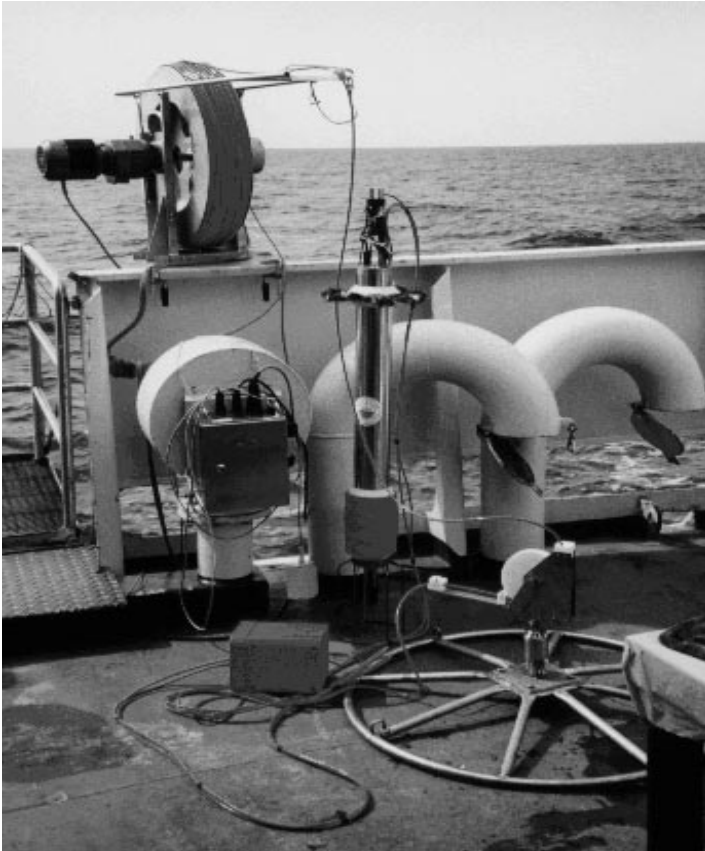
Figure 1: MSS profiler balanced for rising measurements (with red buoyancy rings and ring of brushes) together with the guide pulley
