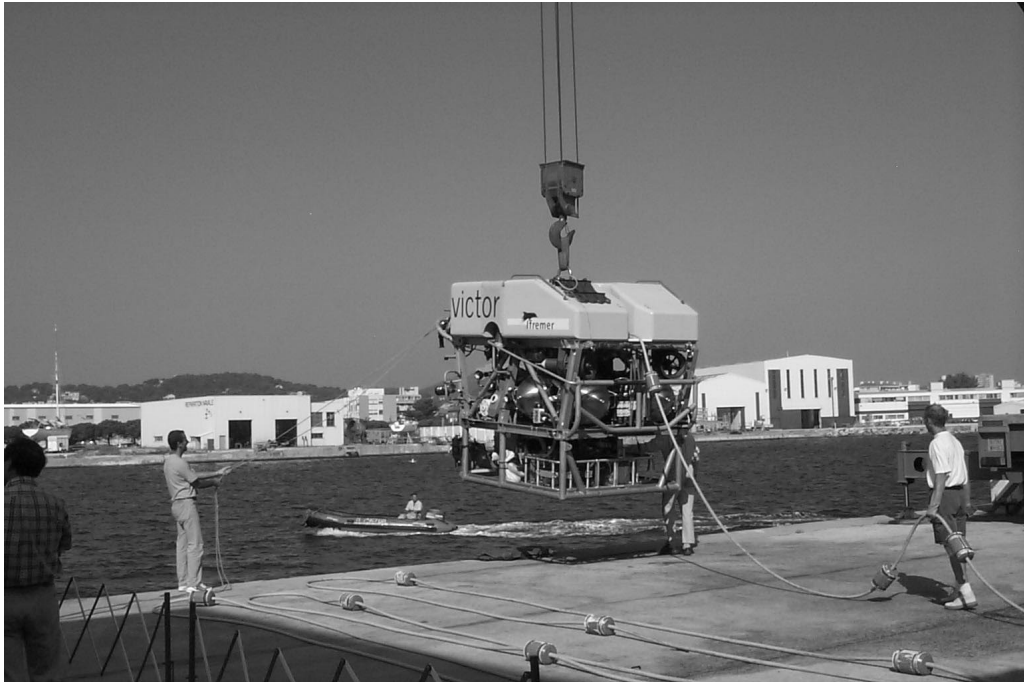
Fig. 2 The ARAMIS tests in Toulon, in May-June 2000. The ARAMIS large skid is fitted under the VICTOR ROV made available by IFREMER
